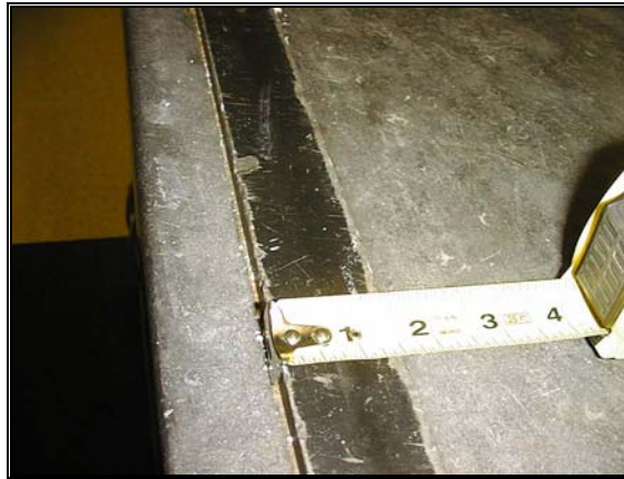
Figure 2 - Work Surface With Perimeter Strip Attached.
